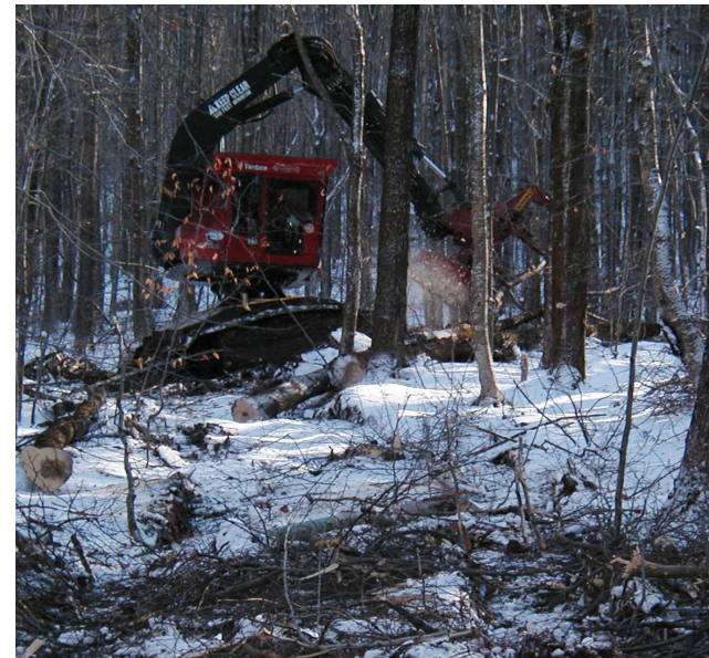
A feller-buncher works on a shelterwood cut designed to regenerate mid-tolerant northern hardwoods on Groton State Forest, VT.
